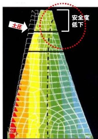
Degraded current cross section
